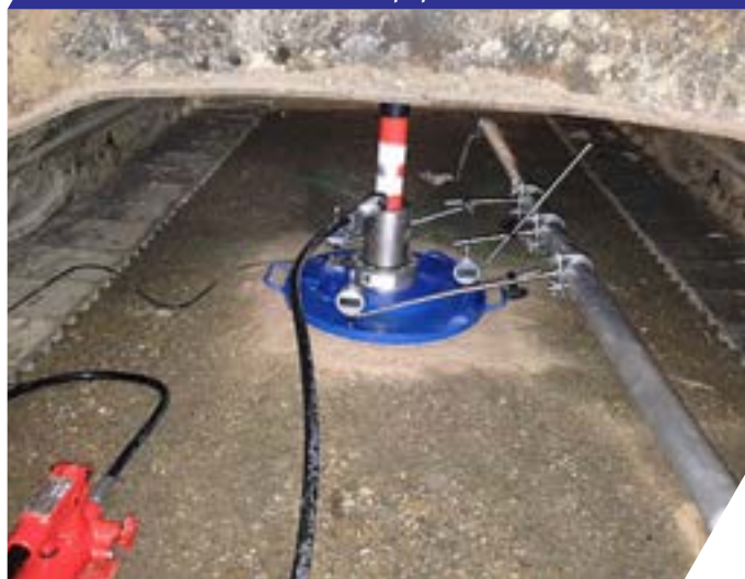
FIGURE 4. Plate Load Test Equipment
