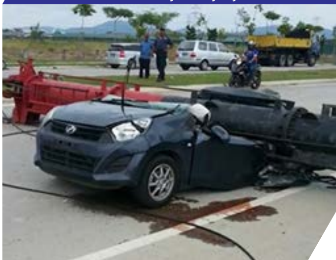
FIGURE 1. Accident Involving a Piling Rig
