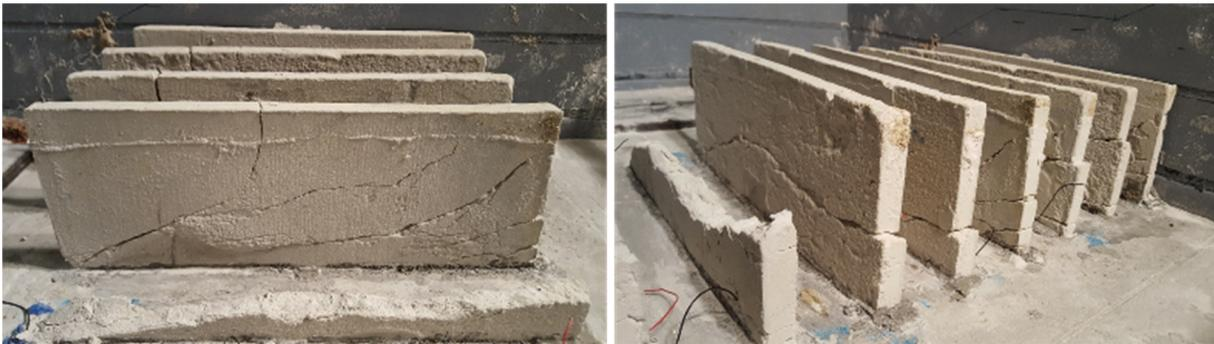
**Fig. 21. Post-test excavation photos of soil-cement panels; toe of berm is to left side of the photos (Boulanger et al. 2018)**
