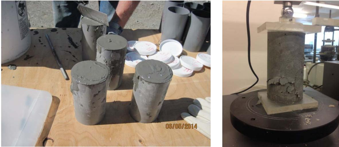
Fig. 34. Testing of field samples: (a) wet grab samples, (b) unconfined compression test
