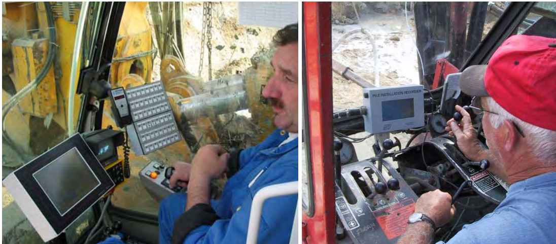
a) Controls on a hydraulic system
