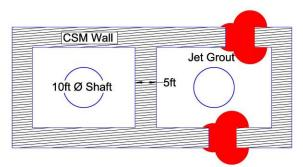
Figure 6: Typical bridge foundation system
