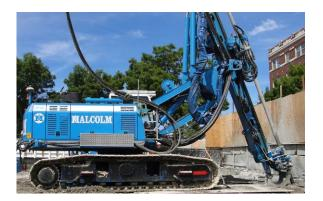
Figure 3: BG 15 inclined jet grouting
