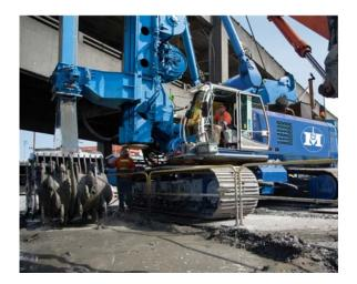
Figure 1: BG 40 with BCM 10, 5 ft wide mixing wheels
