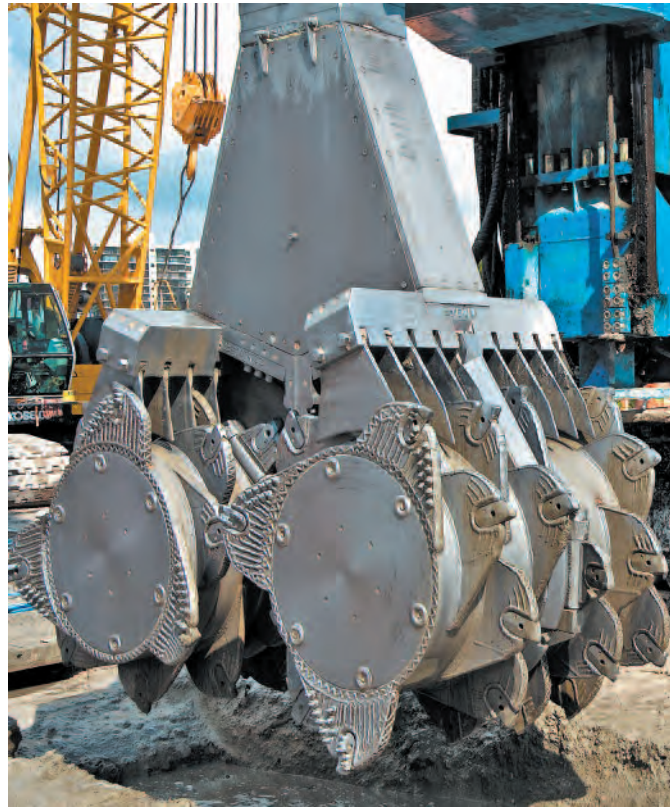
BCM 10 tool for cutter soil mixing.
