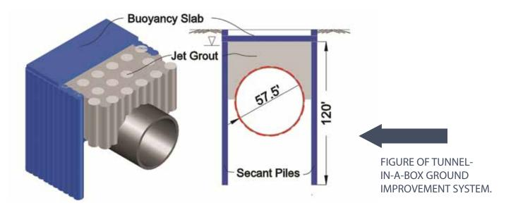
and was locally supported by the pile walls on the box sides, to effectively form a tunnel-in-a-box ground improvement system. The volume inside the box was jet grouted from the elevation of the native glacial materials up to the bottom of the structural buoyancy slab to decrease water pressures and provide the TBM improved ground for tunneling.
