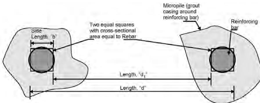
Section Modulus for Composite Structure of Two Equal Squares is equal to
