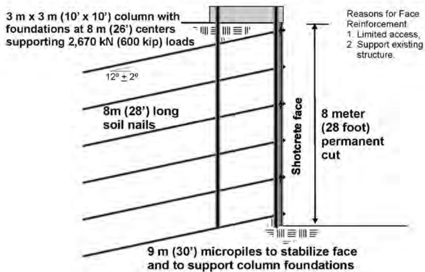
Figure 2b - Micropile Stiffened Face (2006)
