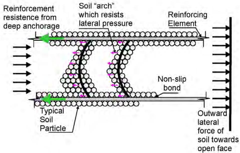
Arching =  $f$  (soil friction, aspect ratio, installation etc.)
