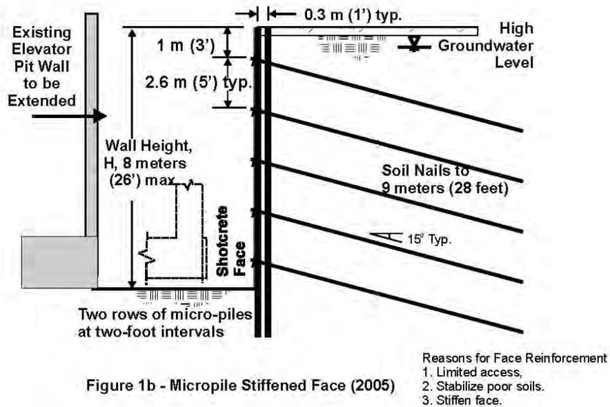
Figure 1b - Micropile Stiffened Face (2005)
