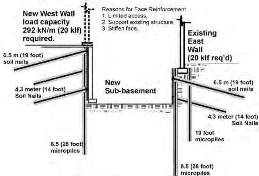
Figure 2a - Micropile Stiffened Face (2005)
