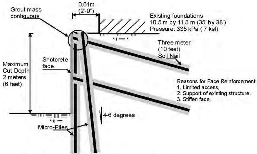
Figure 1a - Micropile Stiffened Face (2004-2006)
