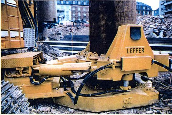
Figure 2. Hydraulic casing oscillator.
