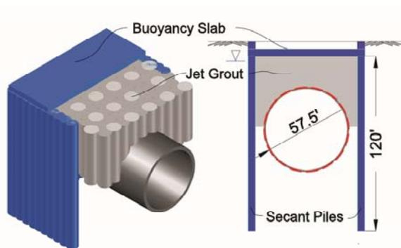
Figure 7: Tunnel Boring Machine ground improvements and horizontal containment
