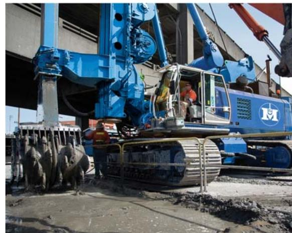
Figure 1: BG 40 with BCM 10, 5 ft wide mixing wheels
