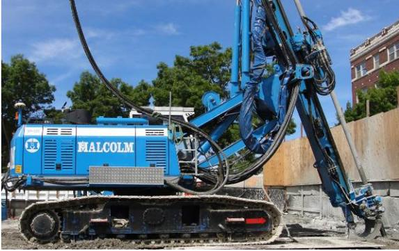
Figure 3: BG 15 inclined jet grouting
