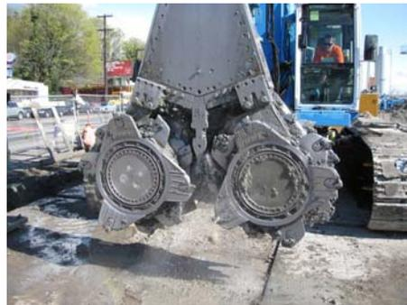
Figure 2. CSM Cutting Head
