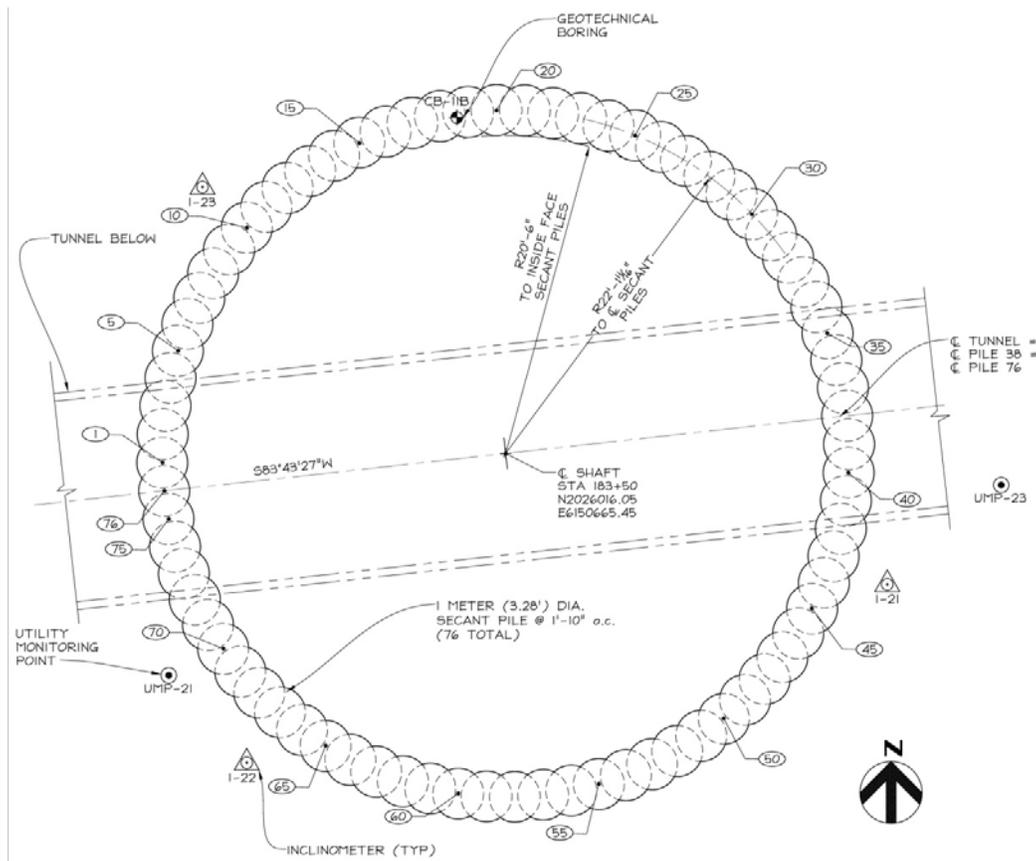
Figure 6: Vargas Shaft Secant Pile Layout
