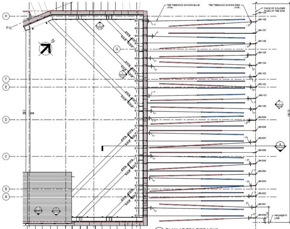
Figure 5: Plan view showing interlaced anchors below 1<sup>st</sup> Street
