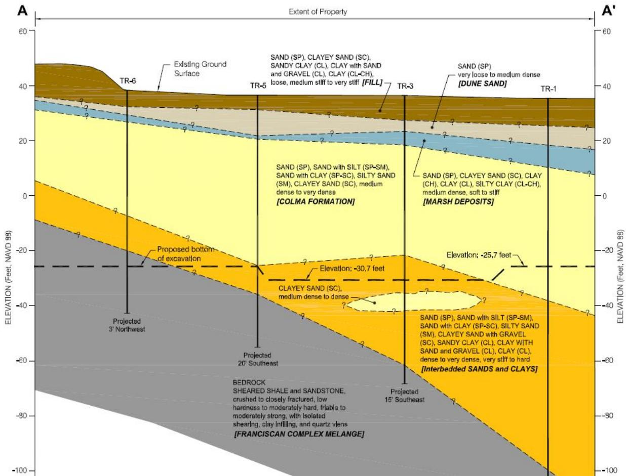
Figure 2: Geotechnical section from SW to NE across site (Langan Treadwell Rollo)
