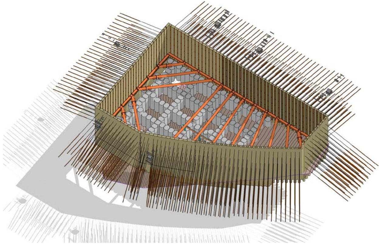
Figure 3: As-designed Support of Excavation Scheme
